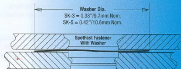
SpotFast fastener with washer installed in sheets.
